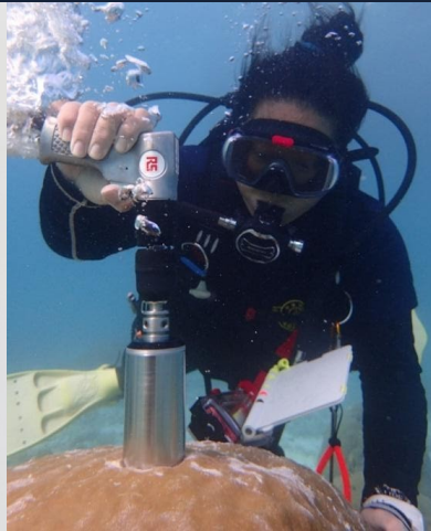
A team member doing pneumatic drilling of a core on a massive coral.
